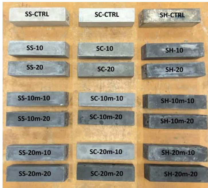
Figure 4. Alkali-activated mortar beams for the Study C.
